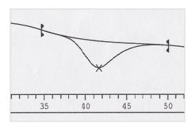
Diagram 1: Typical DSC Profile for PureCol® Collagen with *x* axis = temperature (abscissa) and *y* axis = enthalpy (ordinate)
